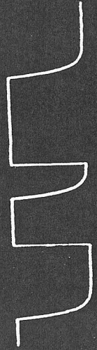
"FM" DISPLAY - FSK TRANSITION ANOMALIES
